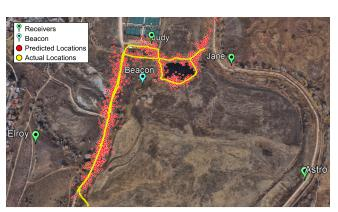
**Figure 1**. Field testing results overlaid on a satellite photo of the test site. The yellow line shows ground-truth GPS measurements while the red dots are positions calculated with our time-of-arrival system. The RMS difference between our system and GPS is approximately 22.6 meters.
