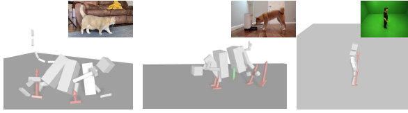
Figure 7: Visualization of ground reaction force. We show the ground contact returned by the simulator. The body part in contact with the ground is colored in red and the ground reaction forces are marked with red arrows. Gravity is represented by a green arrow. Note the contact modes are aligned with the image evidence.
