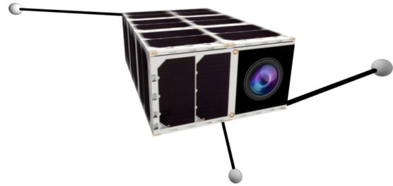
Figure 1. Proposed architecture for a 6U CubeSat space telescope. Each boom has a single degree-of-freedom in linearly independent axes resulting in three-axis attitude control. Magnetorquers are used to desaturate the angular momentum of the booms and keep them within their operating limits.
